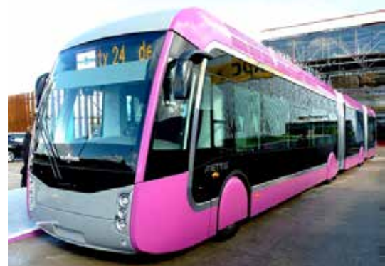
Hibridni avtobus z dizelskim in električnim agregatom https://en.wikipedia.org/wiki/Hybrid_vehicle#/media/File:Mettis_BRT_Metz.jpg
